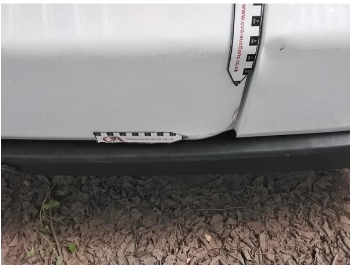
13: Door nsr Dented With Paint Damage
