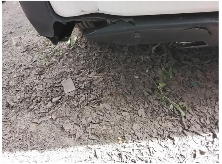
10: Bumper Rear Cracked Over 25mm
