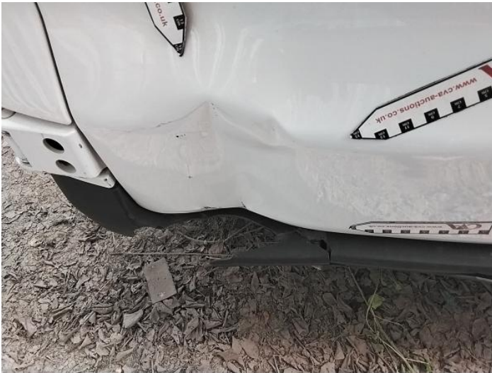
11: Door nsr Dented With Paint Damage
