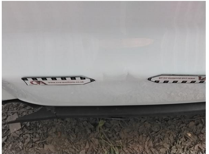
12: Door nsr Dented With Paint Damage
